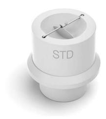
This sensor with Type K Thermocouple reads the temperature of the soldering tip.
